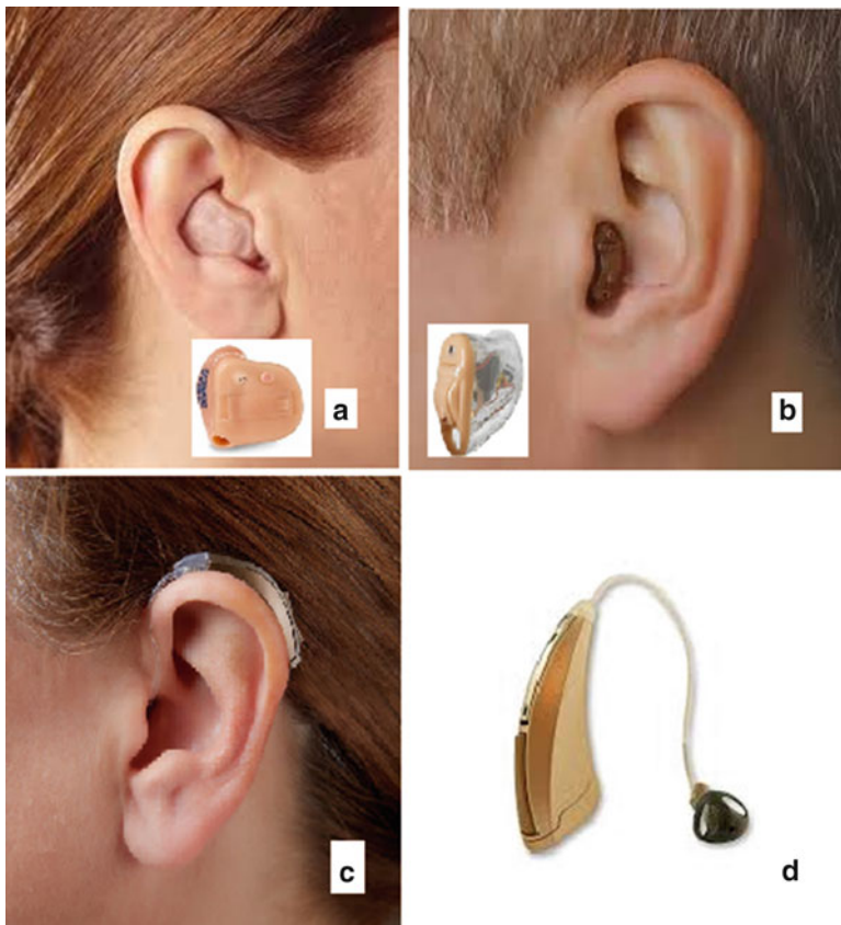
Fig. 1.1 Illustration of some styles of hearing aids. (a) In the ear. (b) Completely in the canal. (c) Behind the ear. (d) Behind the ear with receiver in the canal and open dome
