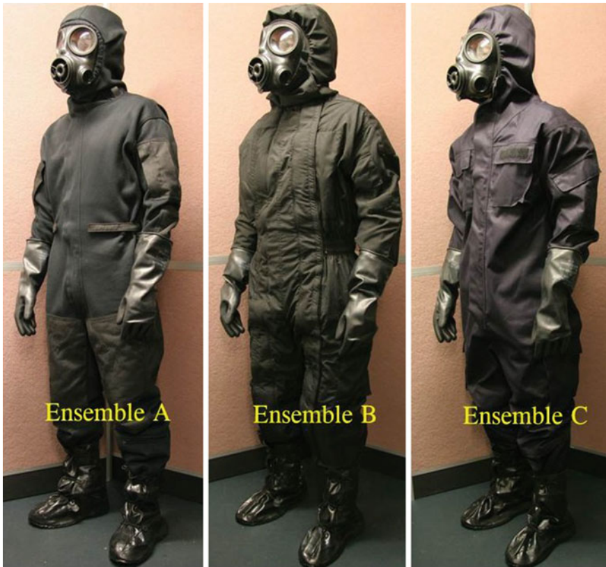
Fig. 10 Chemical, biological and radiological protective ensembles: Ensemble A (Australian low-burden ensemble; CBCS, Melba Industries, Australia), Ensemble B (SWAT, Paul Boye, France) and Ensemble C (CR1, Remploy Frontline, U.K.). Each protective system was evaluated using a standard respirator mask, gloves, over boots, torso body-armor vest and standard military webbing
