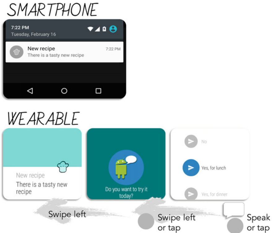
Fig. 16.9 Notification with grammar-based voice response—behavior triggered by the “VOICE NOTIFICATION (GRAMMAR)” button (CookingNotifications app)
