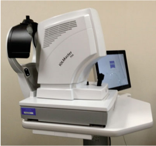
Fig. 11.4 Instrument for measuring length of eye and curvature of cornea
