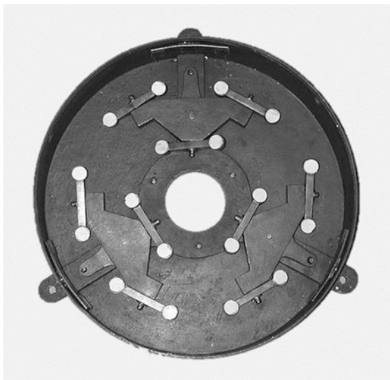
Fig. 4.33 Thomas Grubb’s “whiffle-tree” mirror support for the 15-in. Armagh Cassegrain reflector (1835). Each white pad acts as a contact point. The points are spaced and mounted to three articulating triangles in order to provide uniform load support and so as to minimize flexure of the metal mirror (Image reproduced with permission of the Armagh Observatory)
