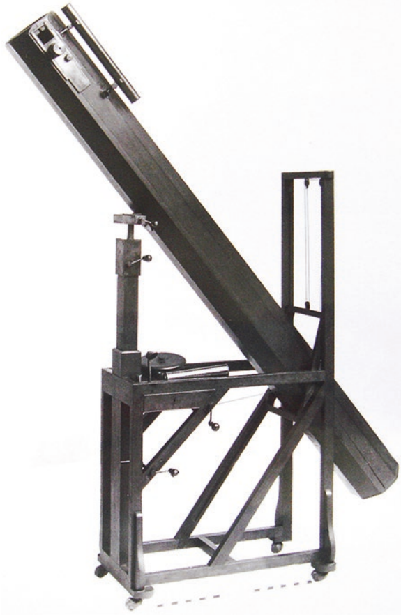
Fig. 4.27 A 7-ft Newtonian telescope by William Herschel, showing the typical lightweight, elegant wooden stand of Herschel’s smaller instruments (Image reproduced by permission of the London Science Museum/Science and Society Picture Library)
