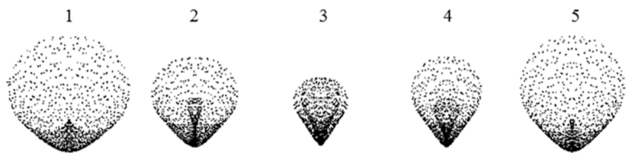
Fig. 4.11 Comatic image flares. These geometrical optics spot diagrams show the faulty ray convergence of an off-axis image point affected by coma. The numbers appearing above the spots correspond to the image plane positions shown in Fig. 4.10. In no case, not even at the best focus (position 3), are the light rays well concentrated
