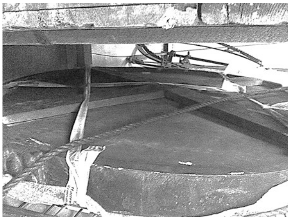
Fig. 4.32 The thicker of the two surviving 48-in. diameter mirrors that William Herschel ground and polished for his 40-ft telescope. Shown above is the rear surface of the mirror revealing the simple support system
