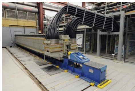
Figure 3. Power feed to Navy laboratory railgun [7].
