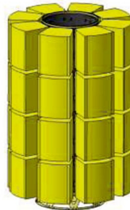
Figure 9 Dispenser configuration for 32 satellite dispenser.
