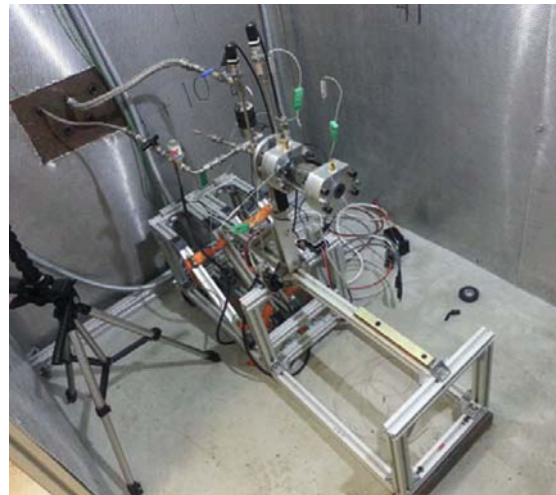
Figure – Instrumented test setup for small 50N class GOx / PMMA hybrid (Kingston University - Wajahat Ahsan)
