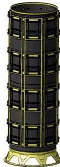
Figure 10 Circular dispenser structure for 32 satellites
