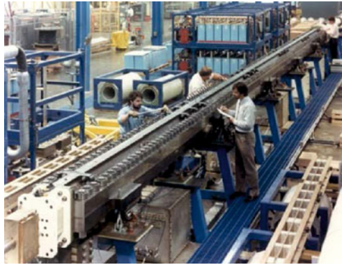
Figure 8. 20-meter long distributed railgun.
