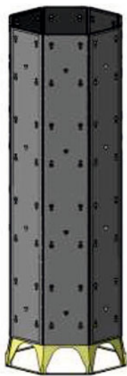
Figure 11 Octagonal dispenser structure for 32 satellites
