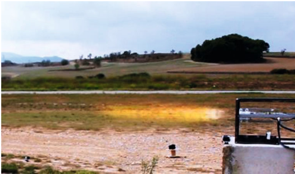
Figure 6: Test of the Teide-0.1 rocket burning propane and oxygen
