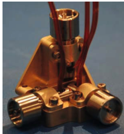
Figure 3. CubeSat-scale reaction wheels. The total height of the assembly is about 3 cm.
