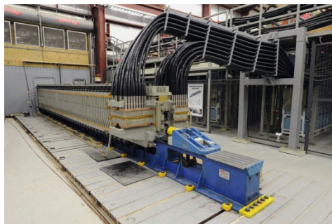
Figure 3. Power feed to Navy laboratory railgun [7].
