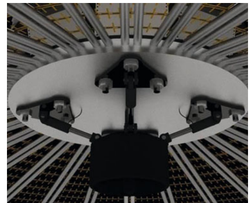
Figure 2-2 Hybrid Plasma Thruster and Thrust Vectoring Assembly
