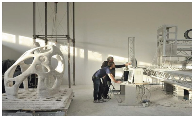
Fig 2. Large Scale Industrial 3-D printing of Building Elements (credit: Edyta Zwirecka)
