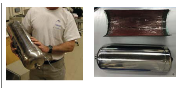
Figure – stainless steel fire extinguisher tank liner and overwrapped sectioned composite tank (Garvey Aerospace, Geodome)
