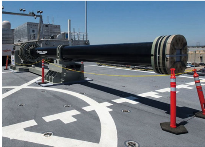
Figure 5. Railgun emplaced on ship deck [8].
