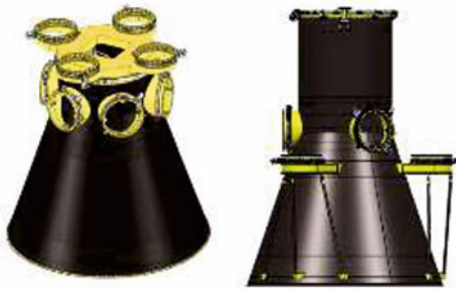
Figure 6 Secondary payload adapter configurations - to the left an additional platform on top for more small sats and to the right an extended version with struts to allow for S/C mounted in a axial position
