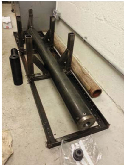
Figure – LOx hybrid rocket engine components (Kingston University – Tim Hodgkinson, Mat Bestelink, Chinonso Ezekwe, Alex Pickard)
