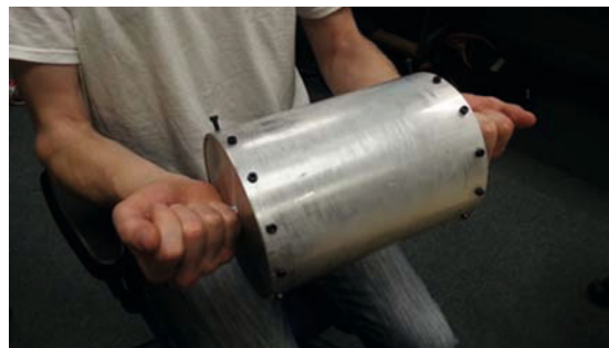
Figure – Prototype N 2 O and LOx oxidiser tank for 200mm diameter test vehicle (Kingston University - Chris Walker, Ben Edgley)
