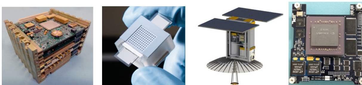
Figure 4: Examples of JPL spacecraft technology development for cubesats/nanosats, and the corresponding mission they will be demonstrated on. From left to right – the deep space transponder (INSPIRE and MarCO), micro-electric spray propulsion (TBD), compact, deployable 0.5 m diameter reflector (RainCube), and onboard data reduction board (M-Cubed/COVE-2)
