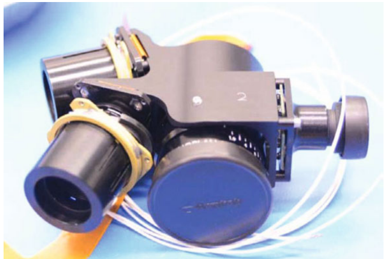
Figure 2. Photograph of the OCSD camera assembly. The two star cameras are on the left.
