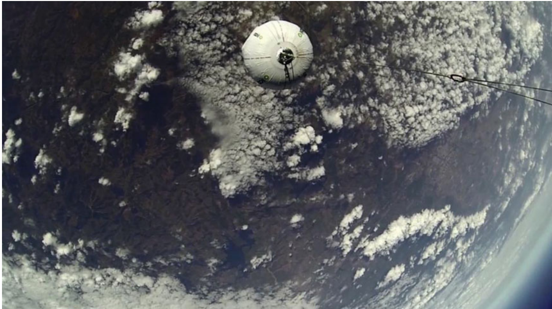
Figure 7: Flexible multilayer tank tested at 27km altitude.
