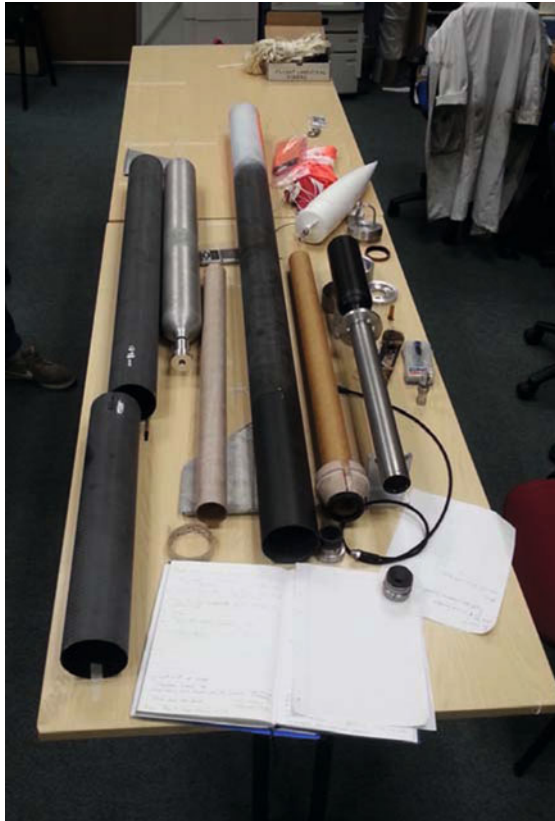
Figure - LATV parts , commercially procured and machined at KU RV campus workshops.
