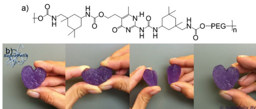
Fig. 10 (a) UPy-functionalized PEG. (b) Self-healing of an UPy-functionalized PEG heart (colored by adding a purple dye, 15 wt% in water): Initial heart shape was reestablished after pressing cut halves together. Figure reprinted and adopted from [61] with permission from SupraPolix BV and John Wiley and Sons (Copyright 2011)
