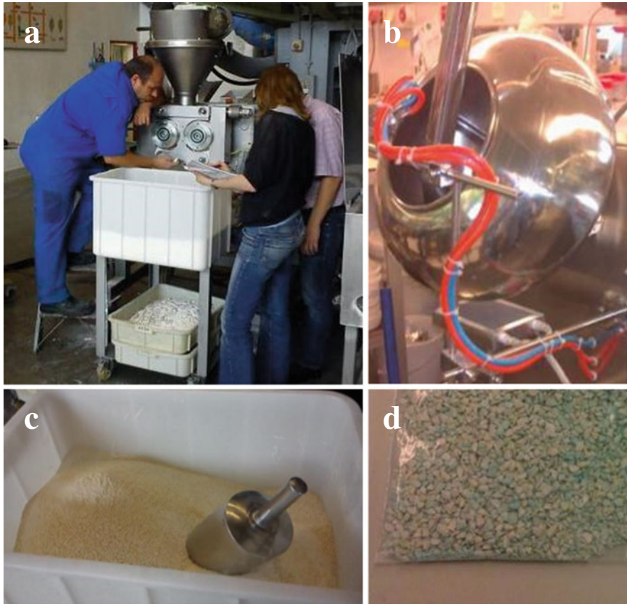
Fig. 11 (a) Roller compaction of powders, (b) coating of particles, (c) uncoated powders and (d) coated powders
