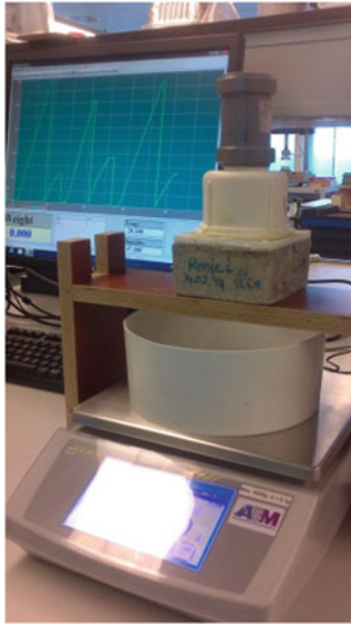
Fig. 14 Left: Set-up for the water leakage test. Right: Residual water flow through cracks at various water curing times. M control mortar, M+HA mortar with healing agent flakes
