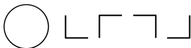
Fig. 1.3 Rotating a circle conveys zero bits of information; rotating an L-shape conveys two bits
