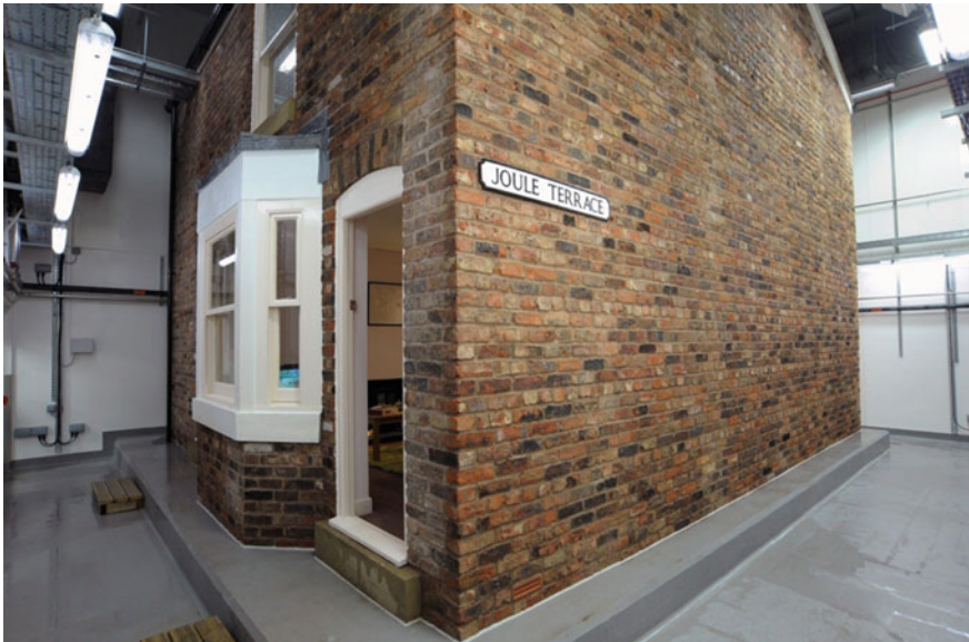
Fig. 7.6 Image of the Salford energy house and chamber
