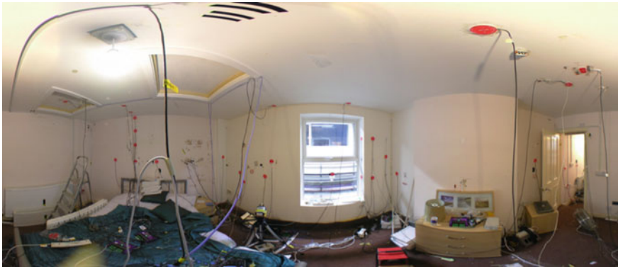
Fig. 7.1 A 360° image of test set up in bedroom one of the test house. Heat flux plates ( red discs ) are positioned on the on the external thermal elements
