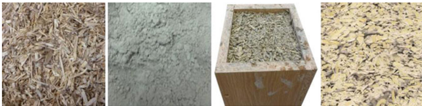
Fig. 16.1 Stages of hemp-lime production: Hemp shiv, powdered lime binder, cast wet material, resultant dried material
