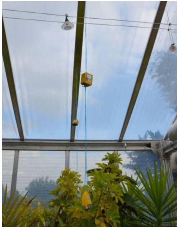
Fig. 5.3 Data loggers installed in the test structure
