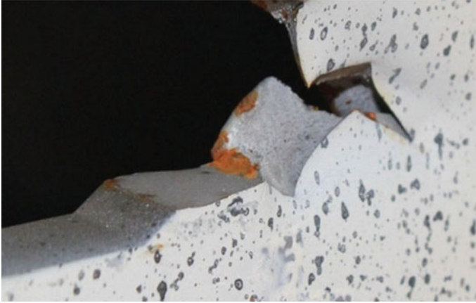
Fig. 8 Crack bifurcation in CT specimen with positive with positive T-stress-induced crack curving T/K = +2.05
