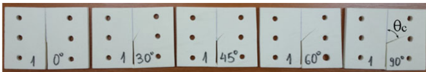
Fig. 14 Crack propagation angle measured on the specimens
