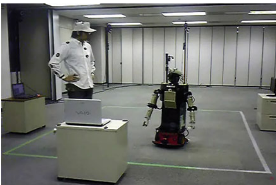
Fig. 72.10 A person and robot implicitly share the target of attention via spatial formation
