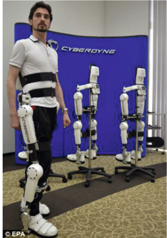
Fig. 64.19 Robot suit HAL-5 designed by Japanese robotics firm Cyberdyne
