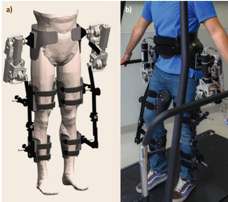
Fig. 64.9a,b EVRYON/LENAR. (a) Wearable robot to assist hip and (b) knee flexion/extension through series elastic actuators (after [64.191])
