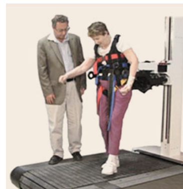
Fig. 64.10 KINE ASSIST for unobtrusive support to patients, allowing them to walk on their own, or with variable levels of support (after [64.200])
