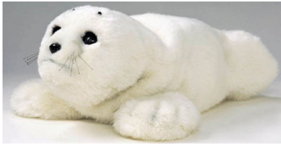
Fig. 64.5 PARO, an advanced interactive robot developed by AIST (after [64.62])
