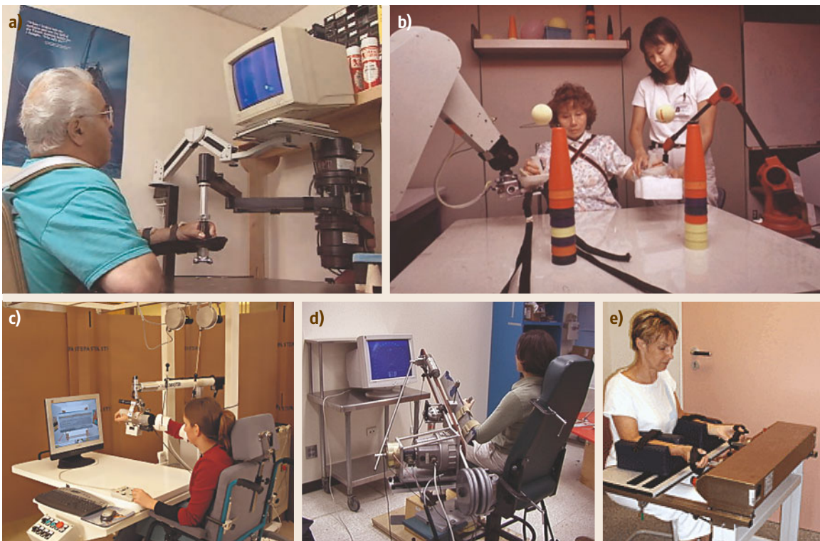
Fig. 64.6a–e Arm-therapy robotic systems that have undergone extensive clinical testing; (a) MIT-MANUS, developed by Hogan, Krebs, and colleagues at the Massachusetts Institute of Technology (USA), (b) MIME, developed at the Department of Veterans Affairs in Palo Alto in collaboration with Stanford University (USA), (c) GENTLE/s developed in the EU, (d) ARM-Guide, developed at the Rehabilitation Institute of Chicago and the University of California, Irvine (USA), and (e) Bi-Manu-Track, developed by Reha-Stim (Germany)
