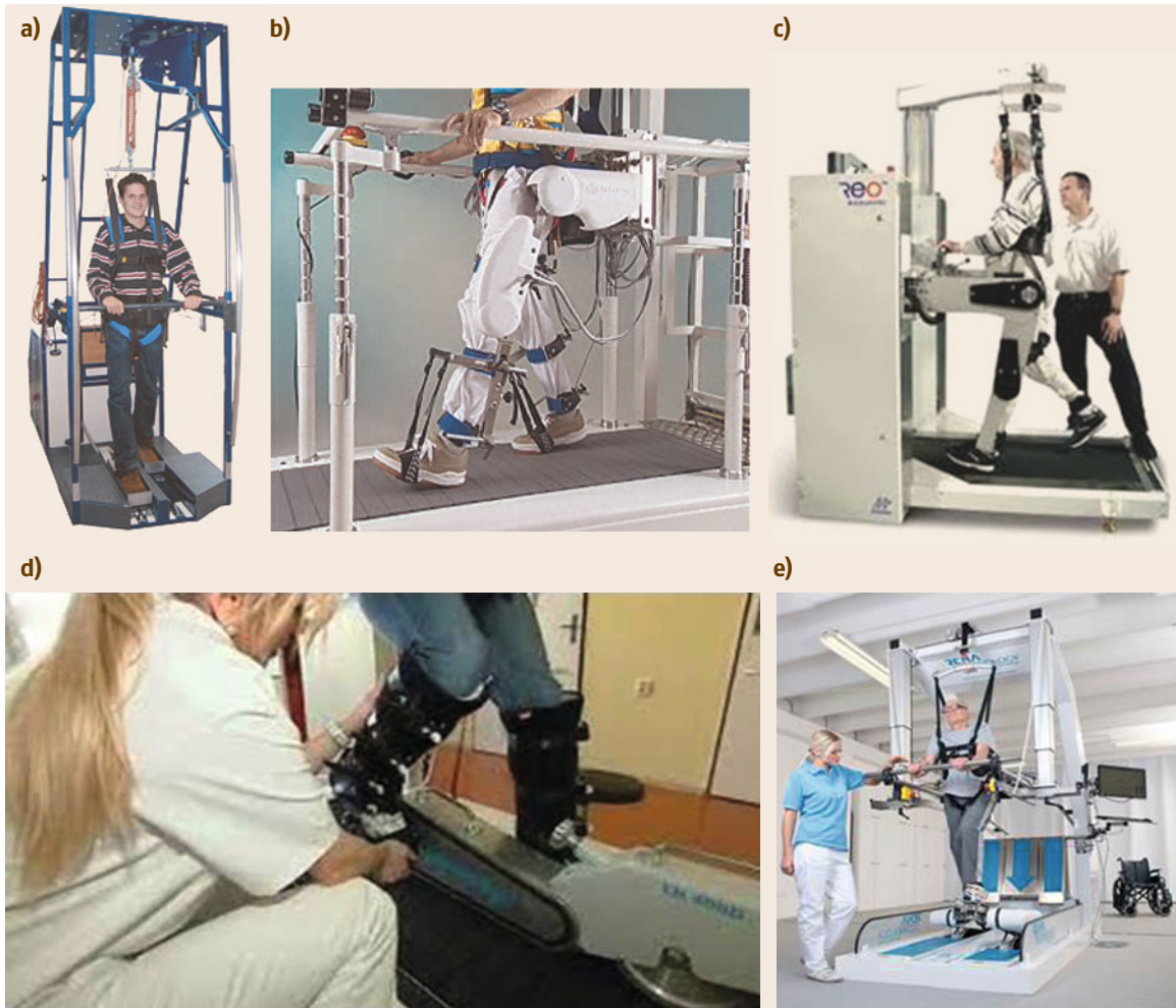
Fig. 64.3a–e Gait-training robotic systems in use in clinics; (a) the gait trainer GT-I, developed by Hesse’s group and commercialized by Reha-Stim (Germany), (b) the Lokomat, developed by Colombo and colleagues and commercialized by Hocoma AG (Switzerland), (c) AutoAmbulator, developed by the HealthSouth Corp. (USA), (d) LokoStation with Lokohelp (Darkov Spa, Czech Republic; after [64.48]), (e) G-EO Evolution (Panos Th. Skoutas S.A., Greece; after [64.49])
