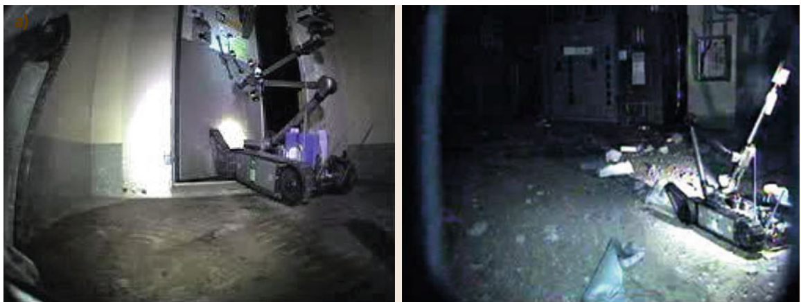
Fig.60.14a,b Operations of PackBots in Unit 1 (courtesy of TEPCO)
