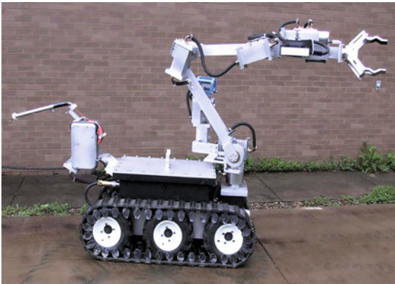
Fig. 60.8 The mine-permissible variant of the Wolverine robot used at the 2006 Sago Mine Disaster (courtesy of the US Mine Health and Safety Administration)
