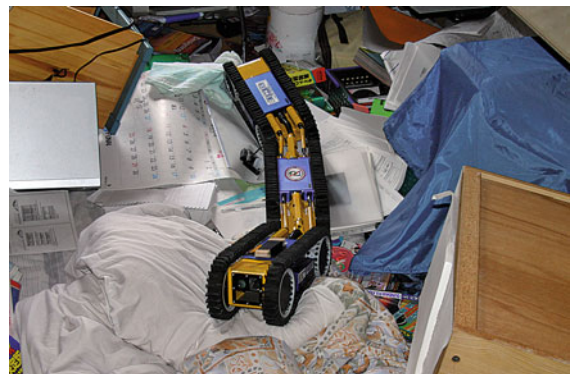
Fig. 60.3 IRS Soryu robot searching a house destroyed by the Niigata–Chuetsu earthquake (courtesy IRS)
