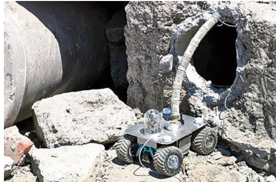
Fig. 60.19 A CMU (Carnegie Mellon University) fixed-base snake being tested at a facility in California (courtesy H. Choset)
