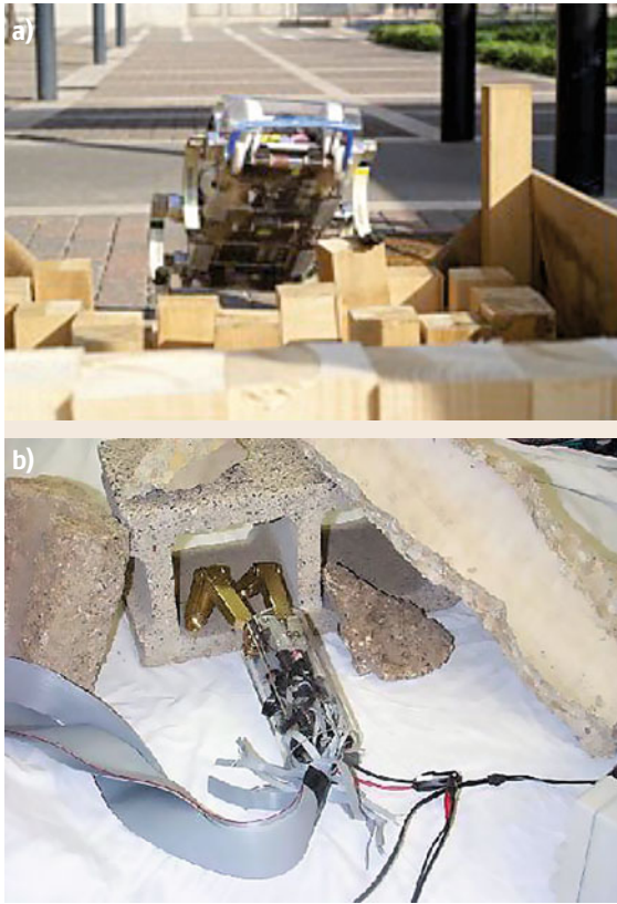
Fig. 60.16a,b Examples of legged and crawler robots. (a) Hexapod (legged) robot from the RHex project traversing a portion of the National Institute of Standards and Technology (NIST) test bed (courtesy of R. Sheh) and (b) Terminatorbot being tested in rescue test bed (courtesy of R. Voyles)
