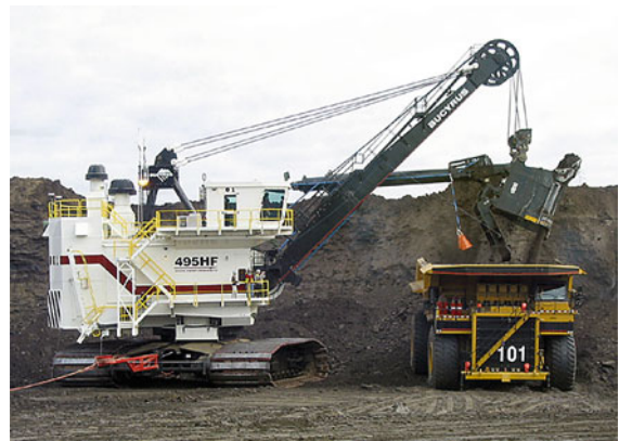
Fig. 59.4 A rope shovel dumping into a haul truck (courtesy of Commonwealth Scientific and Industrial Research Organisation (CSIRO), 2006)
