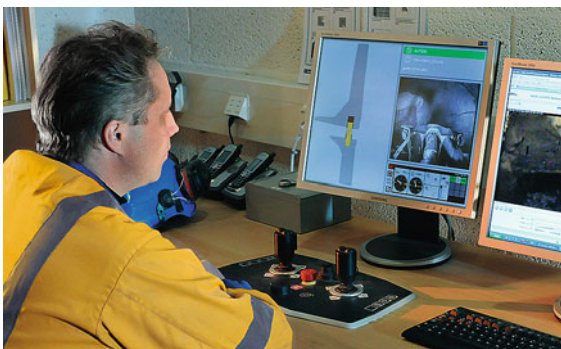
Fig. 59.14 Teleoperator's station for control of underground robotic vehicles at the Kemi mine, Finland (courtesy of Atlas Copco, 2009)
