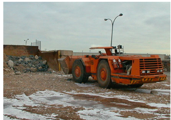
Fig. 59.16 EJC 9T LHD machine conducting robotic excavation experiments in fragmented rock at the engineering facilities of Sandvik Mining and Construction Canada, Burlington, Ontario (courtesy of Joshua Marshall, 2000)
