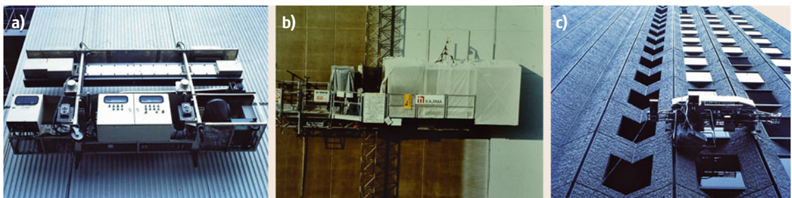
Fig. 57.23a-c Facade painting robots. (a) Shimizu; (b) Kajima; (c) Taisei
