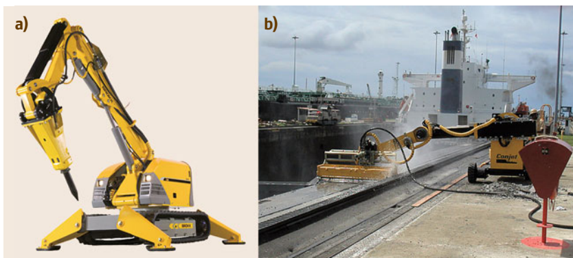
Fig. 57.32 (a) Teleoperated demolition robot (courtesy Brokk AB); (b) water-jet demolition robot (courtesy Conjet AB)
