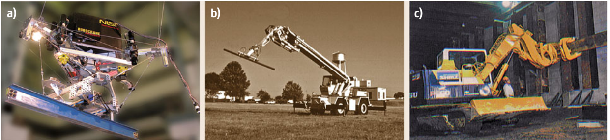
Fig. 57.27a–c Material handling: (a) six degree of freedom robotic crane (after [57.59]); (b) large scale pipe manipulator; (c) large manipulator system (courtesy of Shimizu Corp.)
