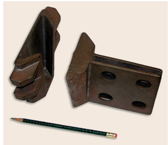
Fig. 57.33 A drop-in, shear-load-only, steel connection
