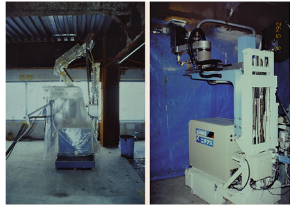
Fig. 57.21a,b Shimizu fireproof coating robots
