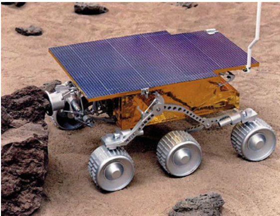
Fig. 55.18 The Pathfinder rover, Sojourner
