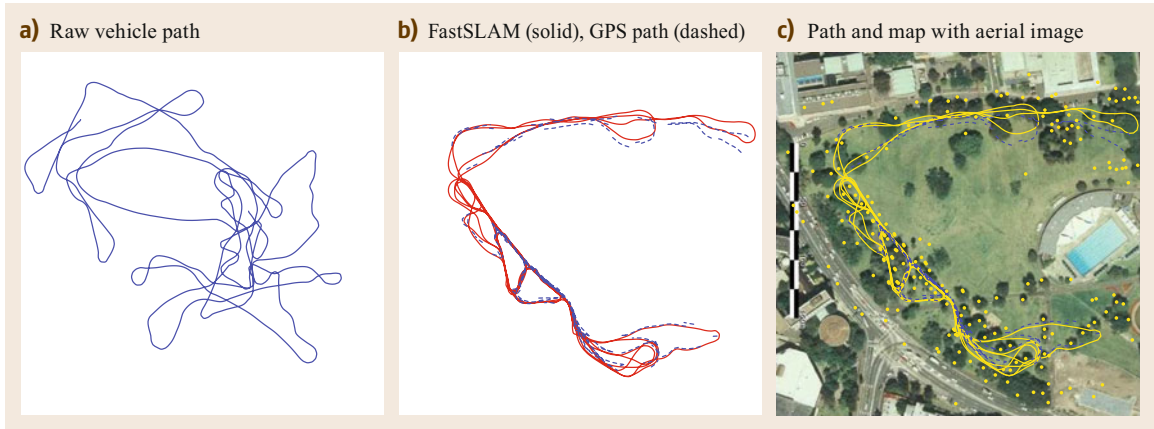
Fig. 46.4 (a) Vehicle path predicted by the odometry; (b) True path ( dashed line ) and FastSLAM 1.0 path ( solid line ); (c) Victoria Park results overlaid on aerial imagery with the GPS path in blue (dashed) , average FastSLAM 1.0 path in yellow (solid) , and estimated features as yellow dots (data and aerial image courtesy of José Guivant and Eduardo Nebot, Australian Centre for Field Robotics)
