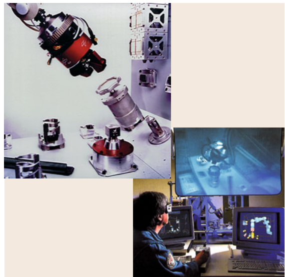
Fig. 43.5 ROTEX, the first remotely controlled robot in space (1993). Telerobot in space and ground operator station (courtesy German Aerospace Center, DLR)
