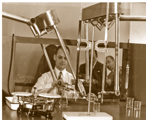
Fig. 43.2 Raymond C. Goertz used electrical and mechanical teleoperators in the early 1950s to handle radioactive material (courtesy Argonne National Labs)
