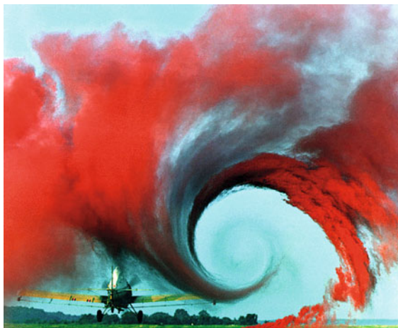
Fig. 26.12 Wake vortex study by NASA at Wallops Island: the tip vortices are visualized using colored smoke rising from the ground
