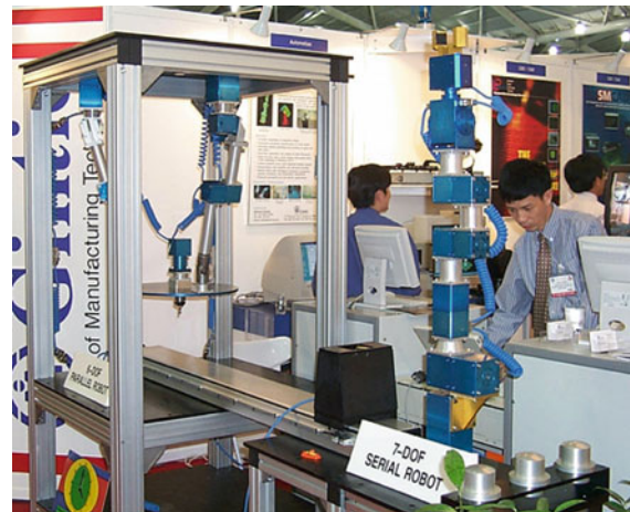
Fig. 22.2 15-axis Reconfigurable Robotic Workcell (after [22.9])
