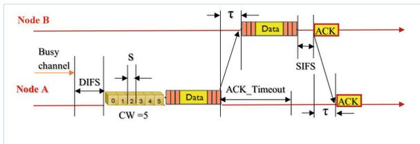
Fig. 5 Different CSMA time durations during DATA/ACK transmission
