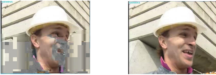
Fig. 12 10-th frame of the received video. Left: video transmission without Raptor codes; Right: video transmission with Raptor codes
