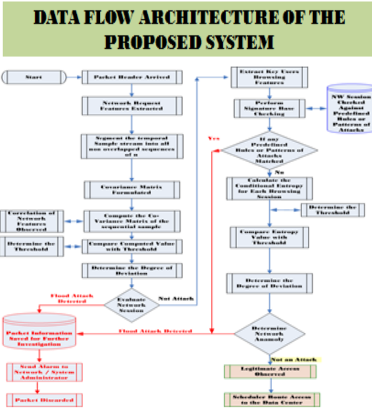
Fig. 4 Data Flow Architecture
