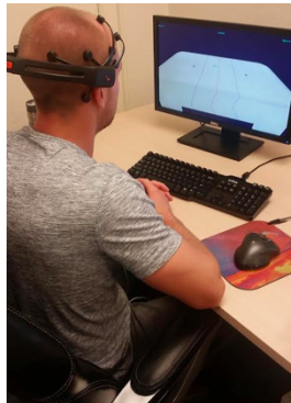
Fig. 4 Player using an EEG headset to interact with the 3D Air Hockey game
