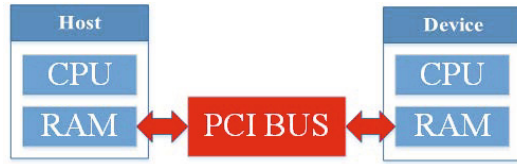
Fig. 1 Heterogeneous CUDA-programming model
