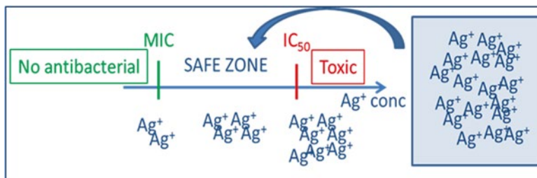
Fig. 10.19 Scheme representing the safe dilution range for applying Ag nanosol samples
