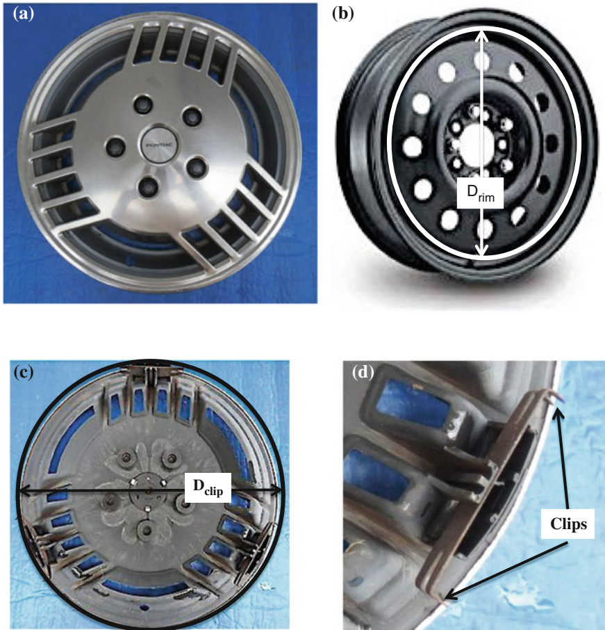
Fig. 2.3 Attachment of hubcap to wheel rim, a Hubcap front, b Wheel rim, c Hubcap back, d Cantilever clips
