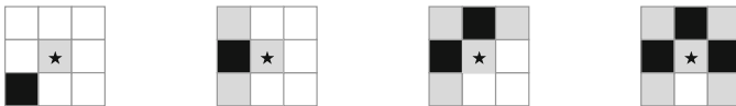
Fig. 1. Base matching templates for characterizing (8, 4) -simple (black or white) points. Notations: each black element matches a black point; each white element matches a white point; each element depicted in gray matches either a black or a white point; each central element marked a ‘★’ is coincident with the investigated point. Note that interior points are non-simple points.
