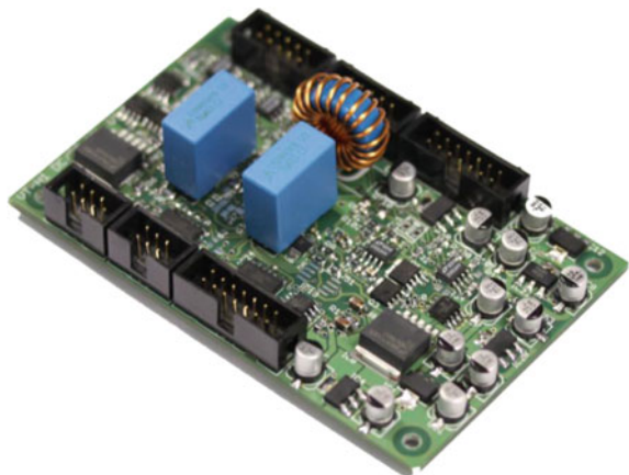
Fig. 5 Simulator board for a single phase of a DC/DC converter
