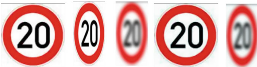
Fig. 3 Simulation of relevant scenarios; from left to right: Original rare sample speed sign; Change of aspect ratio; (Motion) blur; White balance change; Aspect ratio, blur and white balance changes combined
