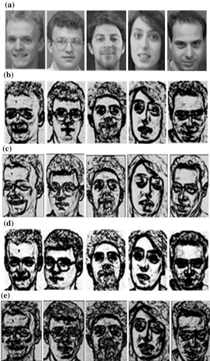
Fig. 5 a Original image, b image with edge detector type 1 morphological gradient, c image with edge detector type 1 Sobel, d image with interval type 2 morphological gradient, e image with edge detector interval type 2 Sobel
