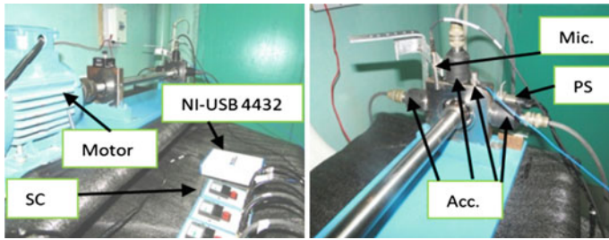
Fig. 1 Experimental setup of ball bearing simulator with array microphone, accelerometers, proximity sensor. * Acc. (Accelerometer), Mic. (Microphone), PS (Proximity Sensor), SC (Signal Conditioner)
