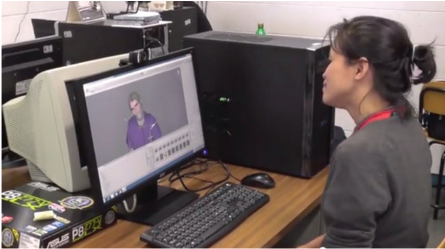
Fig. 4 Avatar: facial and head expressions and movements replicated in real time by the 3D model of a character. The application has been developed using the web service and the facial capture and animation technology of Face Plus [21]. Testing in the CVML laboratory
