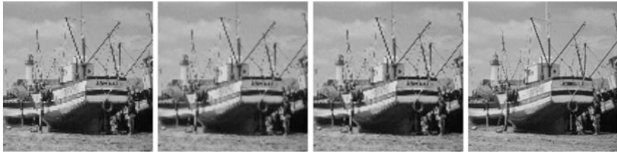
Fig. 9.15 Results of zero, bilinear, bicubic and adaptive interpolation with expanding coefficient 5 for the test image “Boat”
