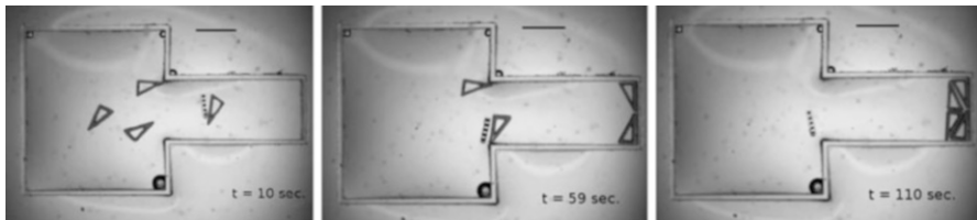
Fig. 4.8 Microscopic view of object manipulation via pushing. The microrobot of type RL3N5 ( 300\ \mu\text{m} wide) assembles four micro-objects (SU-8 triangles, 200 \times 350\ \mu\text{m} ) densely packed into a narrow channel ( 750\ \mu\text{m} wide) within 2 min. The black scale bar is 500\ \mu\text{m} long
