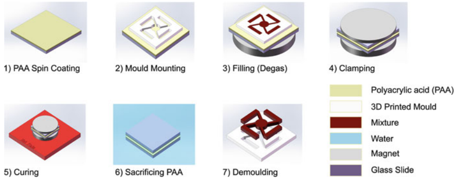
Fig. 28.4 Fabrication process for the actuating plate
