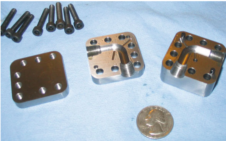
Fig. 18.31 A machined elbow with pressure taps into which the PQT sensor is to be integrated
