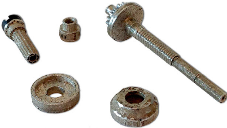
Fig. 3.10 Finished parts (after some considerable rework using a rotary tool)
