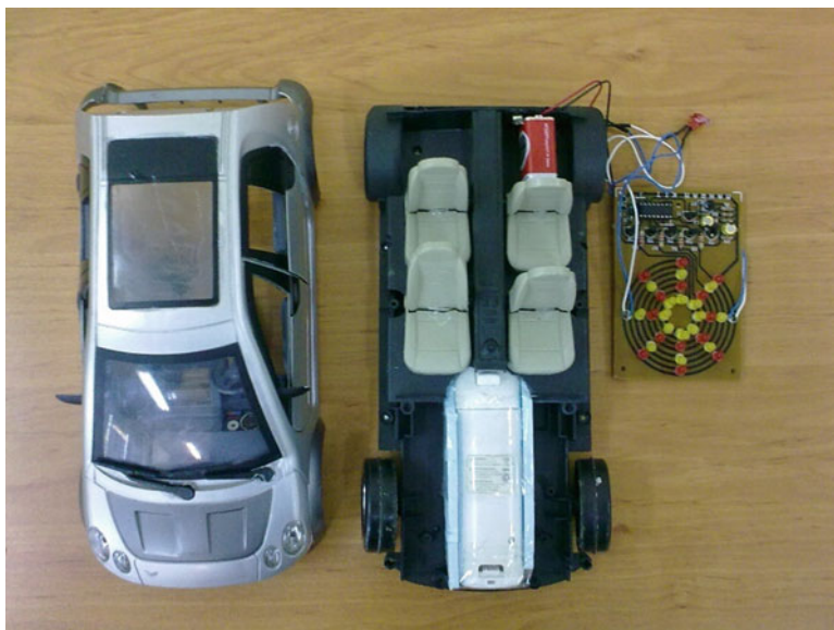
Fig. 13.1 The intelligent toy car equipped with a Nintendo Wiimote to collect acceleration information for screening. The car is equipped with flashing LEDs to make it more attractive for children, especially the children with ASD
