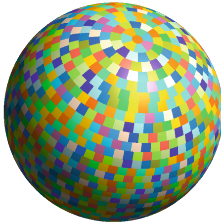
Fig. 3. Equal regions domain decomposition (1600 partitions) for a fine mesh with ~6.6 million nodes (~9 km grid spacing).
