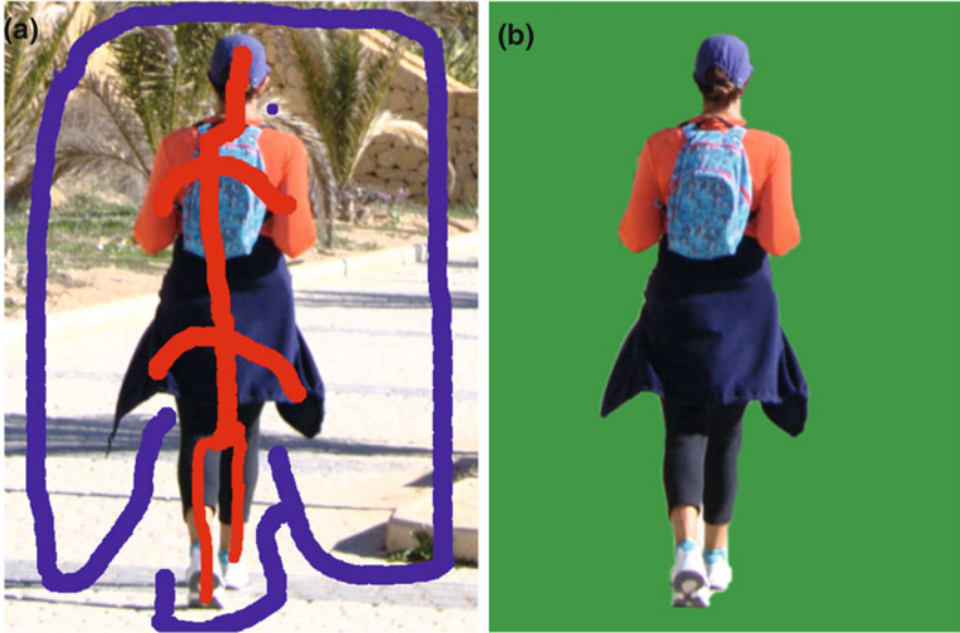
Fig. 3 An example of interactive segmentation. (a) Input image with scribbles. (b) Segmentation result
