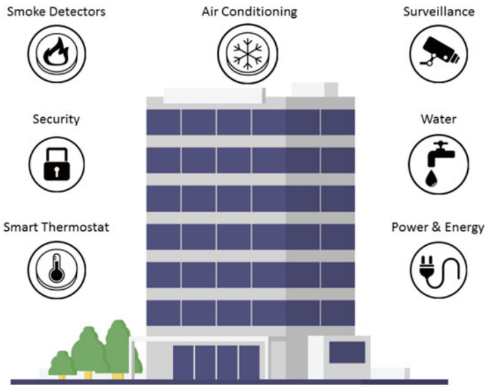
Fig. 2.10 Typical systems controlled by a BAS
