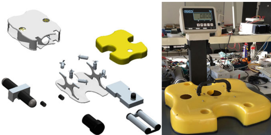
Fig. 2 Measure and calculate mass inertia matrix in PRO/ENGINEER™
