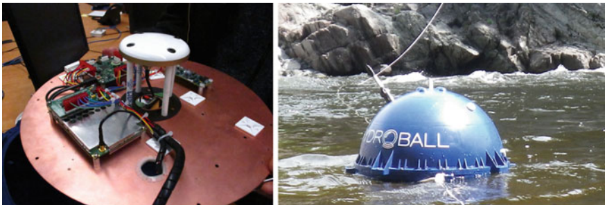
Fig. 1 The HydroBall ® system is integrated in a 40 cm sphere. It is equipped with a SBES operating at 500 kHz, a L1/L2 GNSS receiver and a MEMs Inertial Measurement Unit
