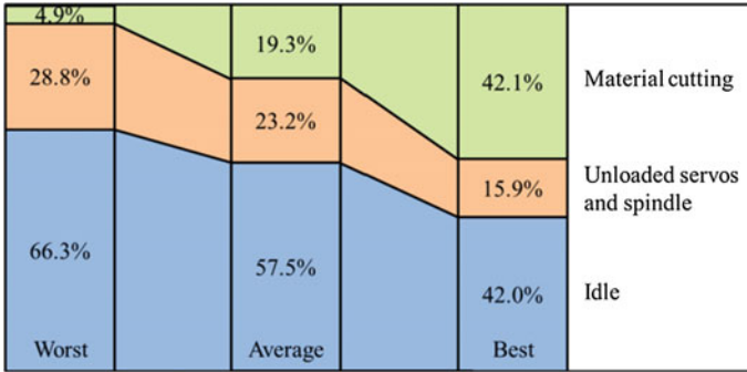
Fig. 7 Dynamic breakdown of the power consumption by Bridgeport VMC 610 based on the results
