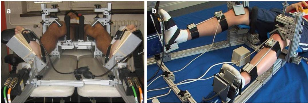
**Fig. 17.3** (a) The knee testing system after the incorporation of motors for force application for consistency. Each patella was also locked into the trochlear groove
