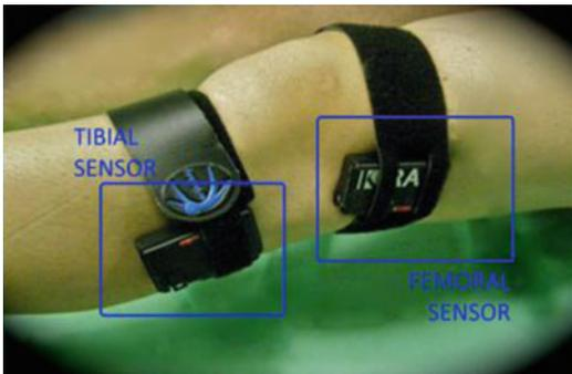
**Fig. 23.6** Example of coupled inertial sensors
