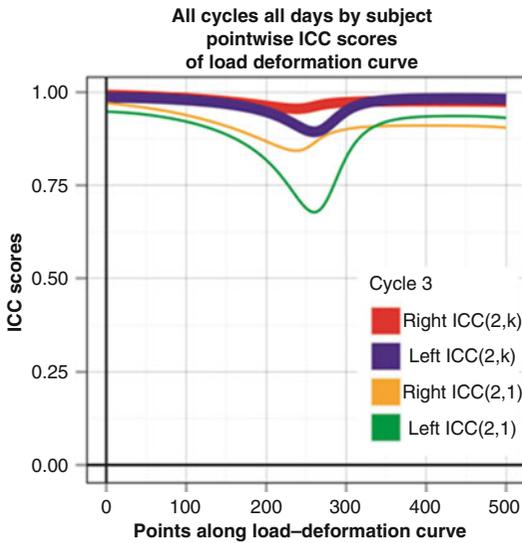
**Fig. 17.12** Average pointwise ICC scores for rotational knee testing performed over 4 days on ten different subjects. ICC scores are significantly lower near torque 0 and position 0, which are near point 250 on the  $x$ -axis
