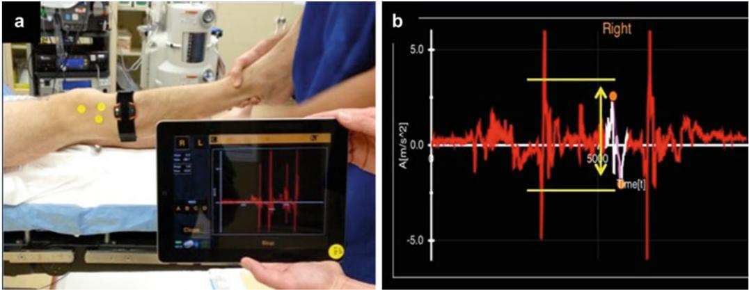
**Fig. 6.3** (a) Up Setup for the KiRA software and the inertial sensors: the sensor is tightly secured in the antero-lateral side of the tibia between anterior tuberosity and Gerdy's tubercle. The axis of the sensor is aligned with
