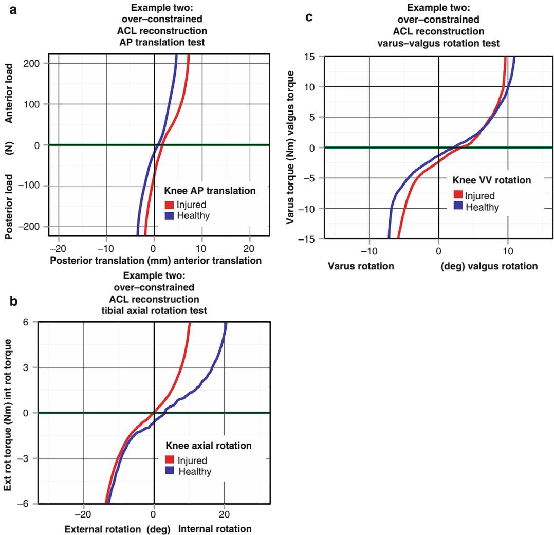
**Fig. 17.14** (a) Anterior/posterior load-deformation curves for the reconstructed and healthy knees showing that anterior/posterior translation in the reconstructed knee was restored to the level of the healthy knee. (b) Tibial axial rotation load-deformation curves for the
