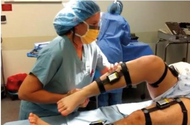
**Fig. 25.2** A pivot shift maneuver being performed on an anesthetized subject with triaxial accelerometers and gyroscopes attached along the tibia and femur of each leg. This placement was used to enable computation of knee
