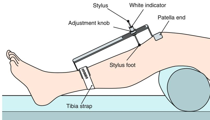
**Fig. 11.7** Rolimeter. This device is centered over the patella and secured to the leg. The stylus is placed over the tibial tubercle, allowing a measurement of translation between the patella and the tibial tubercle
