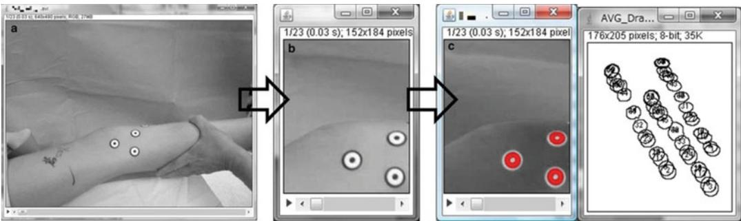
**Fig. 24.2** Processing of images from the video capture undergoing adjustments for grey scale up to the adhesive centroids space location on a XY graph with the use of the “Image J” program
