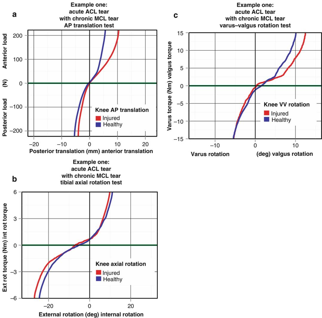
**Fig. 17.13** (a) Anterior/posterior load-deformation curves for the injured and healthy knees showing the increased anterior translation due to an ACL tear in the right knee (red line on the plot). (b) Tibial axial rotation load-deformation curves for the injured and healthy knees. Note that the expected increase in rotation should
