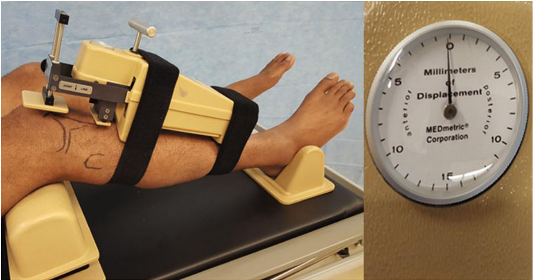
**Fig. 11.4** The KT-1000 positioned on knee of patient with drawn anatomical landmarks (*left*). The analog dial displays the amount of displacement in both anterior and posterior directions (*right*)
