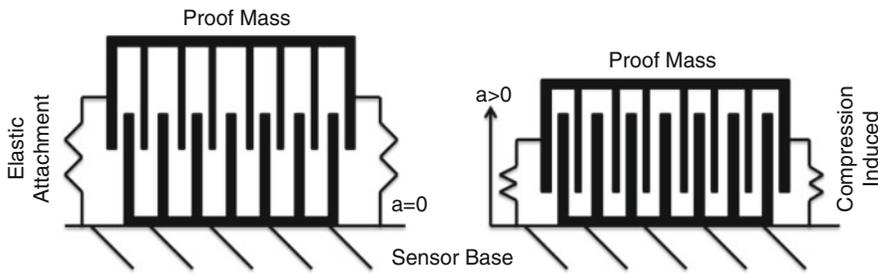
**Fig. 25.1** A schematic representation of one type of MEMS accelerometer. The accelerometer consists of a conductive comb rigidly attached to the sensor base and a second comb-shaped proof mass attached via elastic struts. At the left, with the sensor undergoing zero acceleration, the two combs interdigitate only slightly, resulting in a
