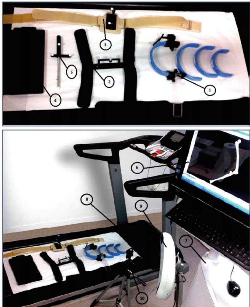
**Fig. 16.1** The KneeKG™ system and its parts. 1. Femoral harness (4 interchangeable arches), 2. tibial harness, 3. sacroiliac belt, 4. feet position guide, 5. pointer, 6. computer, 7. cart, 8. treadmill, 9. video camera, 10. reference body
