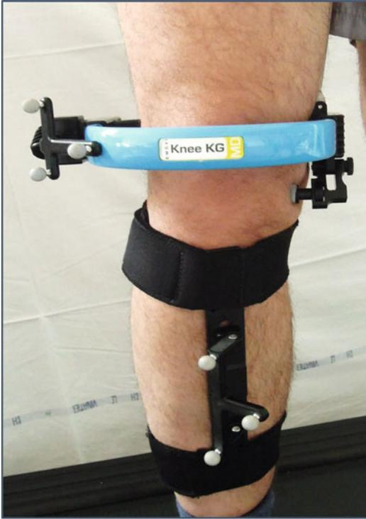
**Fig. 16.2** Anterior view of a right knee fitted with the KneeKG™ tracker system
