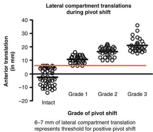
**Fig. 21.3** Lateral compartment translations during pivot shift in the different pivot shift grades (Reprinted from Bedi et al. [5] with kind permission of Springer Science and Business Media)
