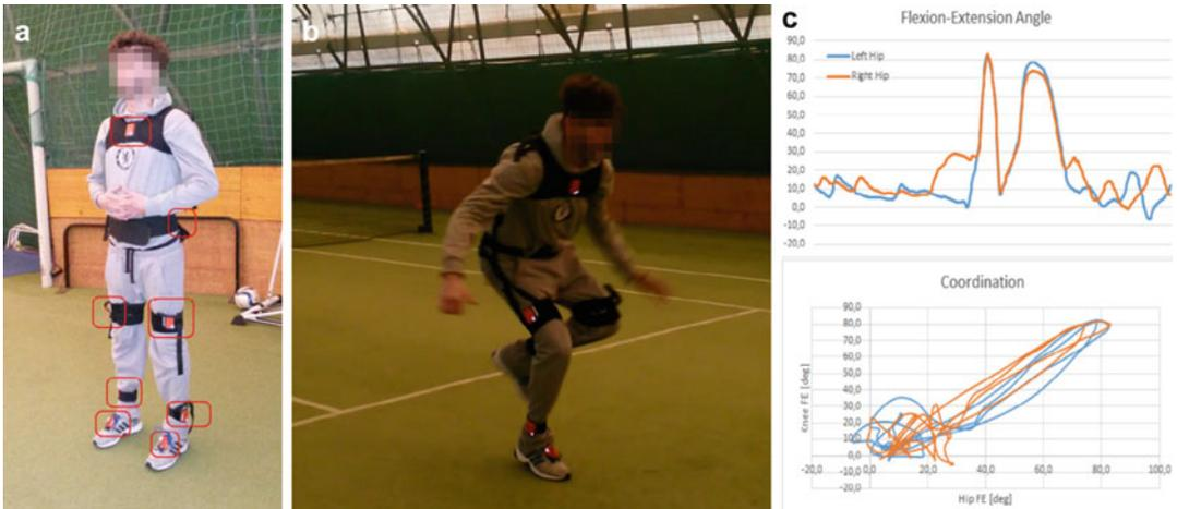
**Fig. 42.10** (a–c) The Xsens system (Xsens Technologies, NL) used during field acquisition (Courtesy of Isokinetic, Bologna, Italy): (a) static calibration, (b) landing after a
