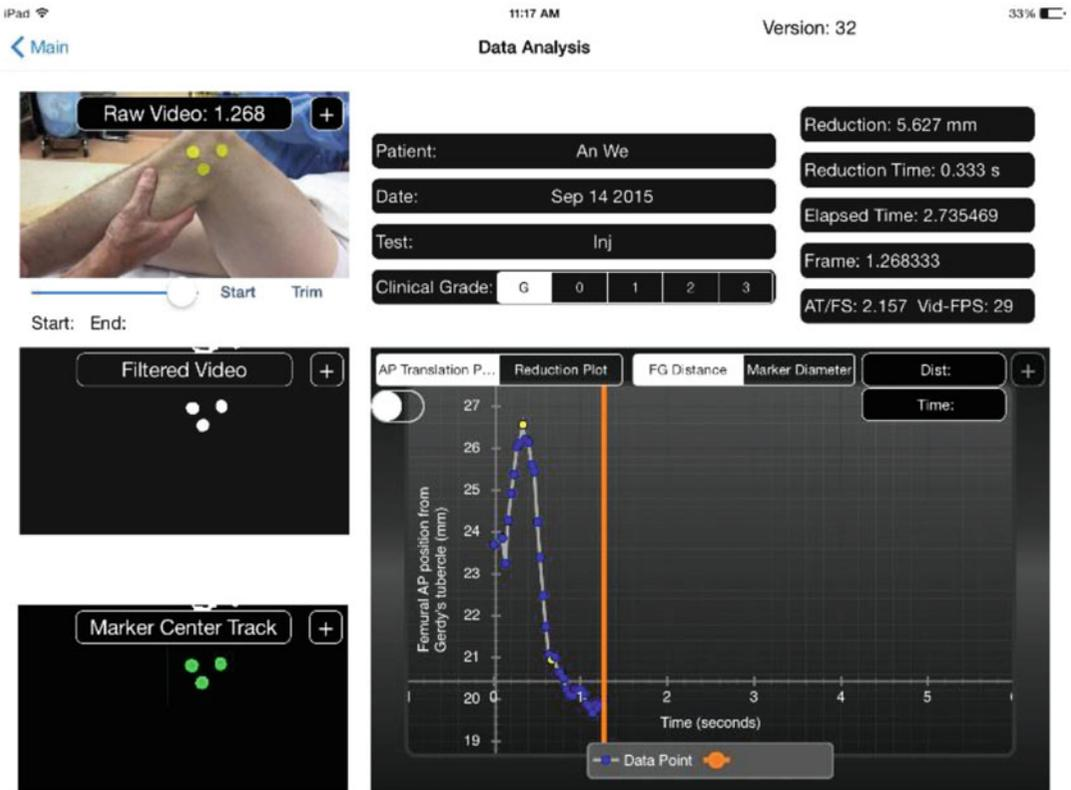
**Fig. 24.6** iPad application screen. The video of the pivot-shift test appears on the top to the left; the tracking of the markers is shown below the video. The anteroposterior femoral translation starting from Gerdy's tubercle (in mm) per time (in seconds) is shown on the graph
