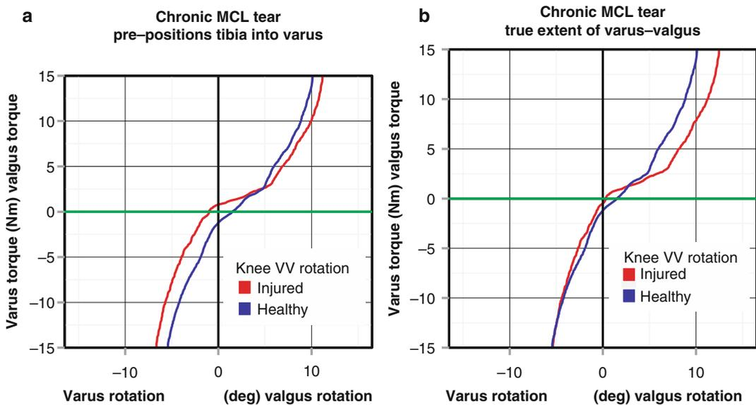
**Fig. 17.9** (a) A load-deformation curve in a patient with a chronic MCL tear. (b) The load-deformation curve after normalizing to the initial position. The MCL tear becomes obvious after this preprocessing step
