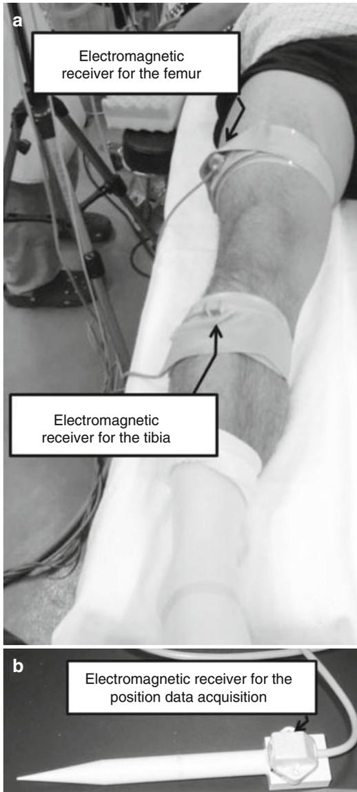
**Fig. 22.1** Electromagnetic sensor setup. (a) Two sensors are attached onto the thigh and the lower leg. (b) Third receiver is attached to the original styler which can be used to digitize the 3D position data of bony landmarks
