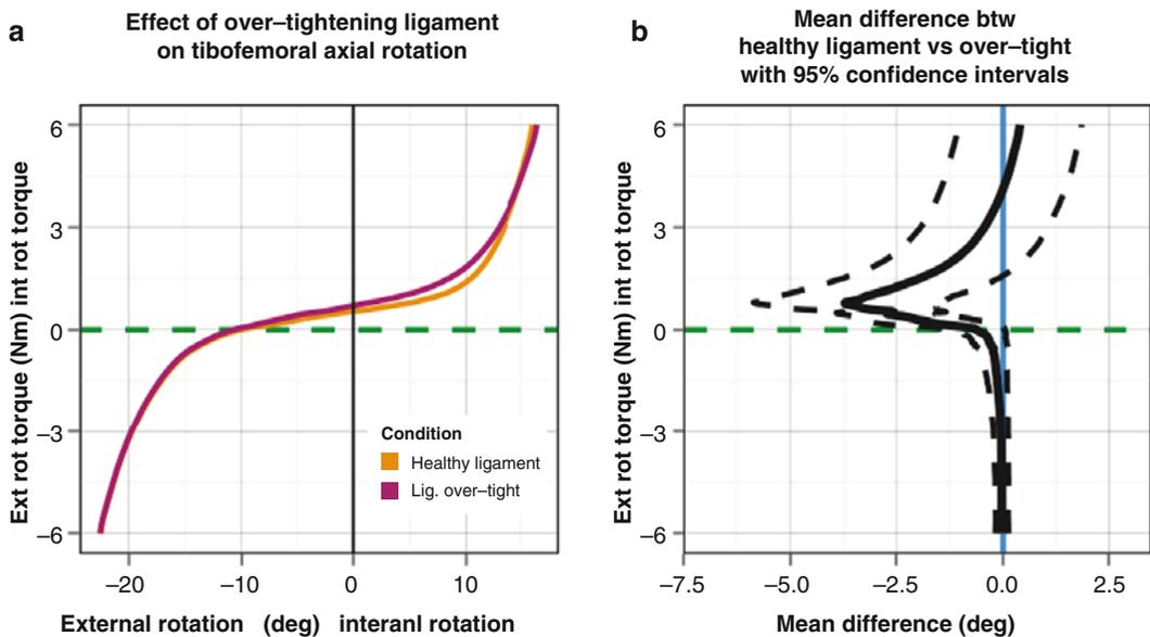
**Fig. 17.10** (a) Load-deformation curves for two conditions. (b) A pointwise curve comparison with 95% confidence intervals (dashed lines). Note the difference in the extent of the curve near 2 Nm. In the difference curve,
