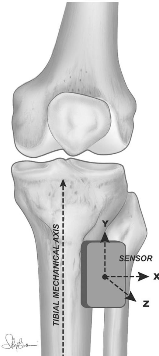
**Fig. 42.4** Positioning of the KiRA (Orthokey LLC, DE, USA) device. X, Y, Z are the three axis along which the acceleration measurement is performed
