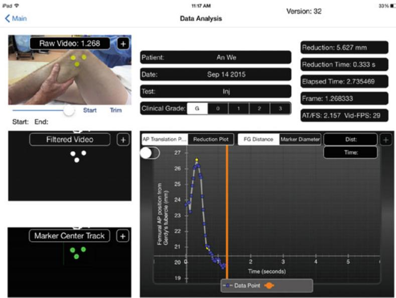
**Fig. 42.5** Configuration of skin markers and display of software interface for PIVOT application for the iPad. A pivot shift test is performed in the photograph on the upper right with skin markers placed on the lateral femoral condyle, Gerdy’s tubercle and the fibular head. Tracking of the skin markers as observed on the iPad interface is shown in the two lower left boxes prior to and during the performance of the pivot shift. The change in the anterior-posterior
