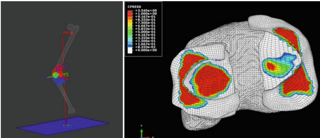
**Fig. 42.9** Dynamic RSA data processing: bone position and ground reaction force (*on the left*). Finite element (FE) simulation of the stresses on the tibial cartilage and menisci (*on the right*)
