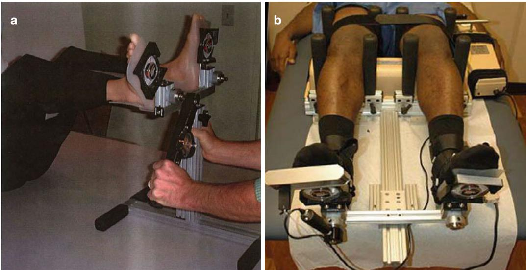
**Fig. 17.1** (a) The first rotational knee testing system utilized manual application of force and visual reading of a goniometer. (b) The next version of the knee testing sys-
