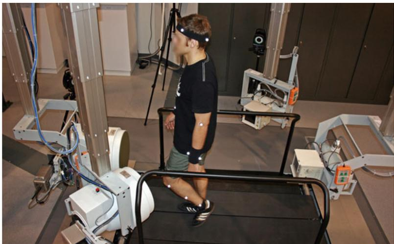
**Fig. 4.1** High-speed stereoradiographic imaging system with instrumented treadmill, University of Pittsburgh. Biplane images are acquired simultaneously at up to 180 frame/s
