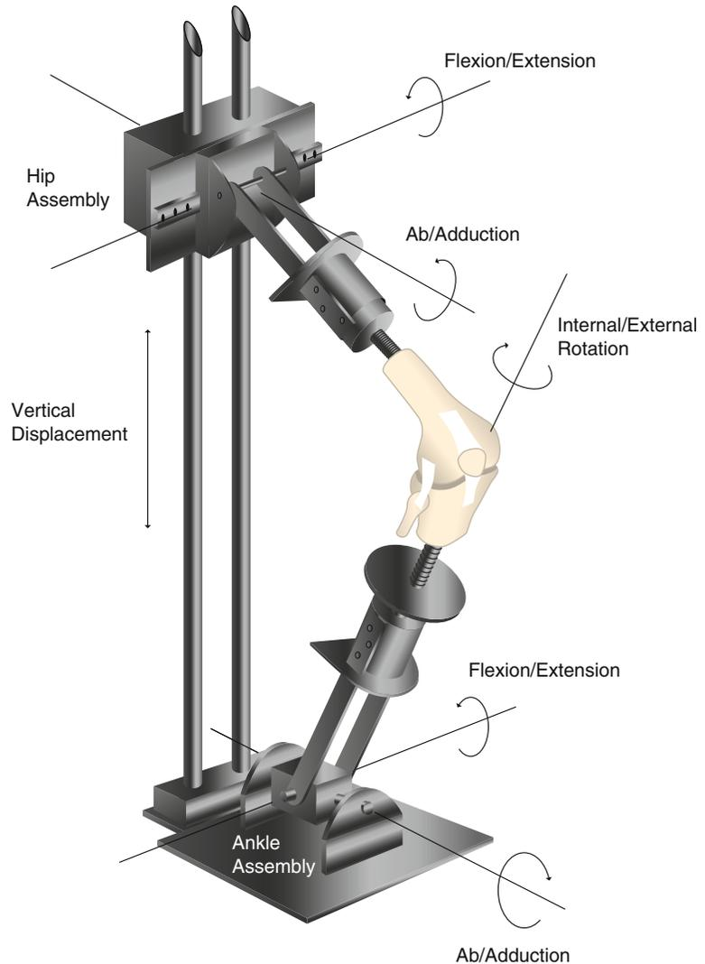
can be applied to simulate body weight by holding assemblies from the hip unit. The rig is used to simulate stance activities with knee flexion, such as the motion during riding a bicycle, rising from a chair, or climbing stairs [87].
