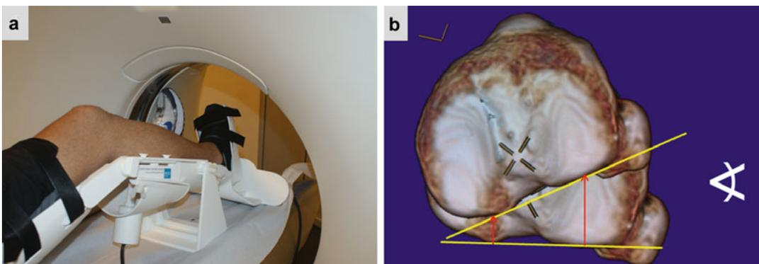
**Fig. 5.3** Porto-knee testing device (PKTD<sup>®</sup>) inside MRI equipment (a); CT 3D axial view representation of tibial internal rotation and anterior translation after load application by the PKTD (b)
