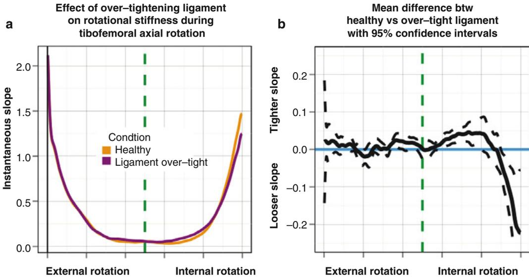
**Fig. 17.11** (a) A first-order derivative curve calculated from the original load-deformation curve showing stiffness characteristics of a normally reconstructed ligament and an over-constrained reconstructed ligament. (b) A pointwise
