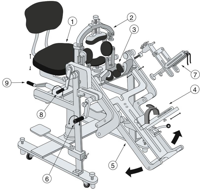
independently. Knee flexion angle was adjustable, though recommended at  $20^\circ$ . The patient reclined to allow muscular relaxation. The tibia was controlled by a clamp just below the tibial tubercle, and anterior and posterior forces were applied to the tibia manually by a lever connected to a gear system. Displacement was amplified by a gear system, quantified by a strain gauge load cell, and then fed into a computer to produce a graph.
