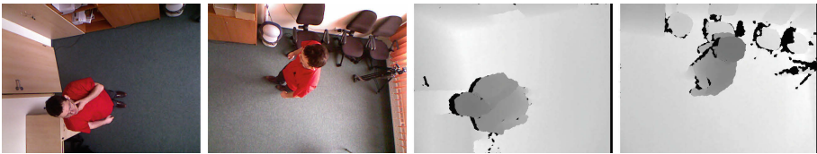
Fig. 2. Example top-view images captured by Kinect mounted on pan-tilt head, RGB images (top row), depth images (bottom row).
