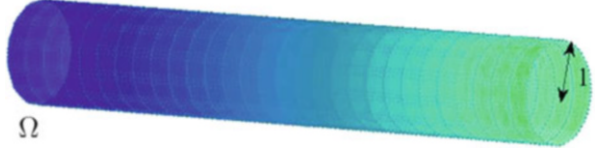
Fig. 2 Reference domain after the change of variable, we obtain a cylinder of radius one
