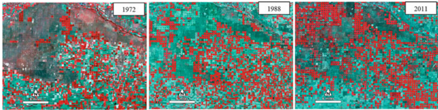
Fig. 3.4 Change in irrigation system type in southwest Kansas as shown by the change in field shapes from square to circular over the 3 years of 1972, 1988 and 2011 (image source: http://www.nasa.gov )
