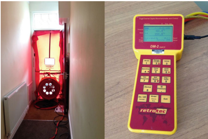
Fig. 11.10 Equipment used for air permeability tests
