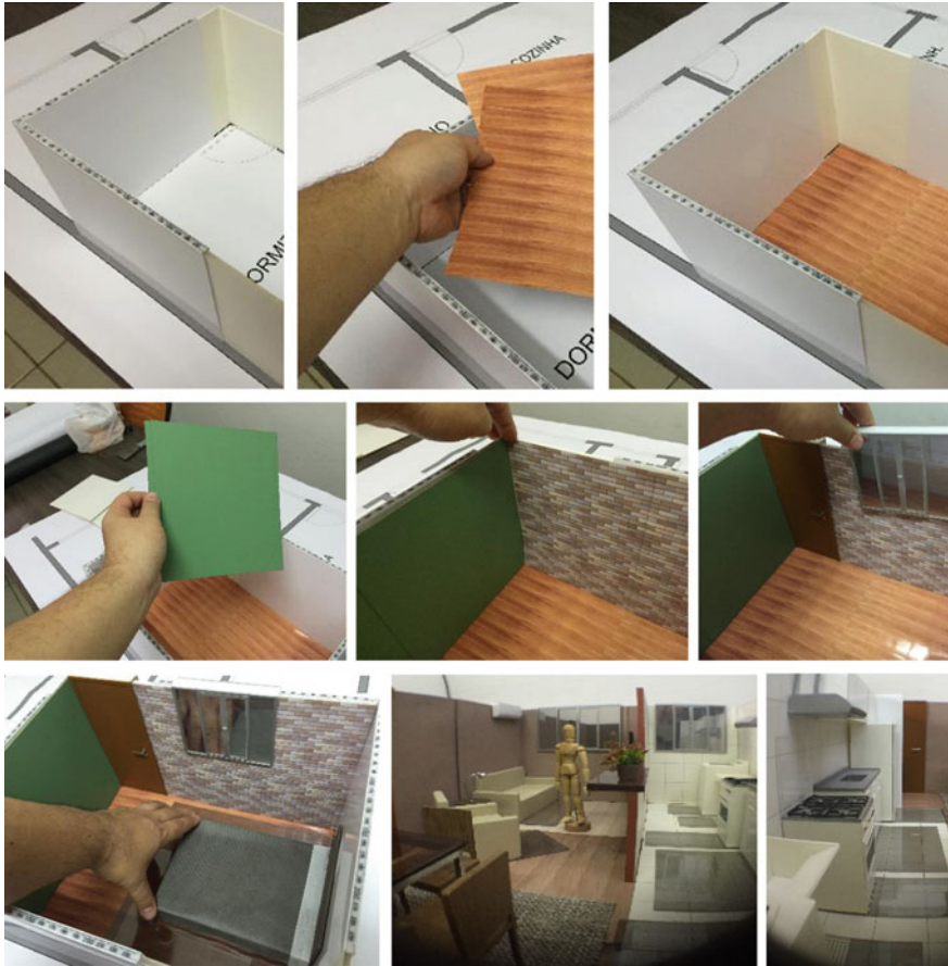
Fig. 4.2 An adjustable physical housing model for mass customisation
