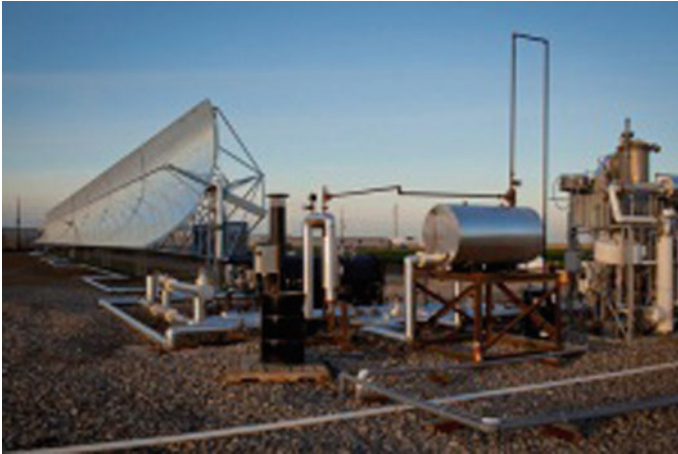
Fig. 9.5 Solar thermal desalination system (Woody 2015)
