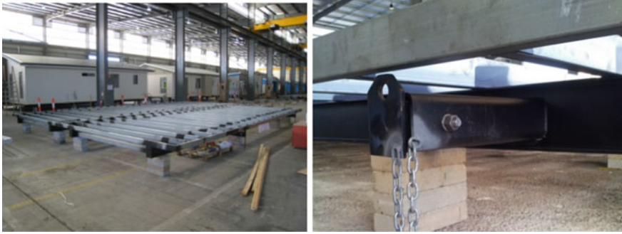
Fig. 3.11 The factory line is a static production line with each chassis blocked up from a factory floor. The right image shows a retractable lifting arm that accommodates bottom and top lifting mechanisms as required for the building type and site conditions
