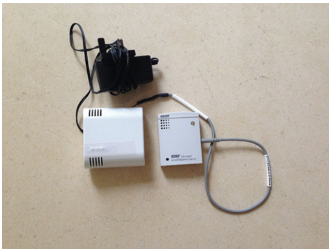
Fig. 11.12 HOBO U12/12 data logger (right) and CO 2 sensor (left) assembly
