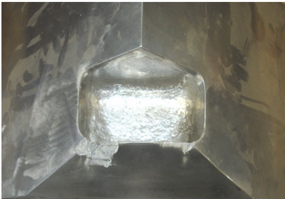
Fig. 4.5 Protection shelter in the form of a washbasin and the material damage because of the impingement of water-droplet strings
