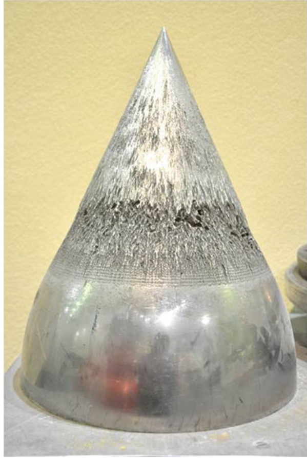
Fig. 22.1 Sand abrasion on the surface of an injector needle after 165 operating hours (Photo KWO)
