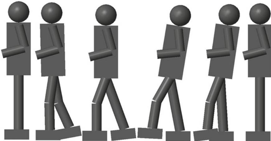
**Fig. 9** A single step of the biped robot. The robot moves from *right* to *left* as the time passes
