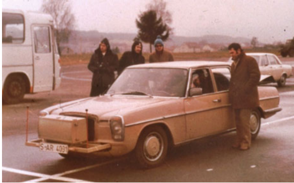
Fig. 10.3 16 GHz automotive radar system built by SEL (Standard Electric Lorenz) 1975. Source: private collection of the author
