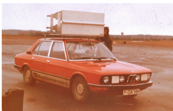
Fig. 10.2 10 GHz automotive radar system built by VDO, early 1970s. Source: private collection of the author
