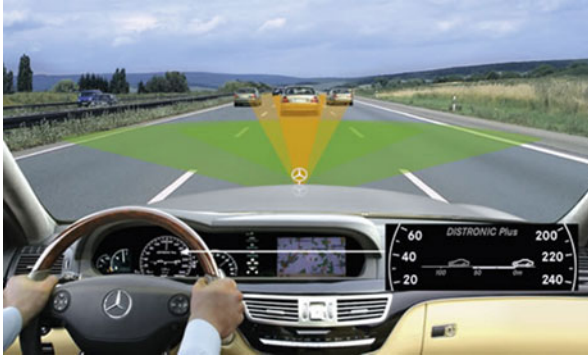
Fig. 10.7 Antenna configuration schematic of “Distrionic Plus”—combining LRR and SRR for urban employment ( yellow : 77 GHz LRR-Sensor, green : 24 GHz SRR-Sensor). Source : Daimler AG, Stuttgart, Germany
