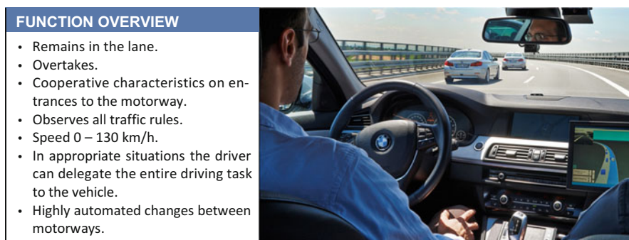
Fig. 15.2 Function overview—Highly Automated Driving on the motorway
