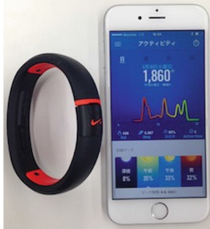
Fig. 1. The Nike+ FuelBand SE is a device meant to be worn on the wrist. The client application presents graphical output produced by the data from the FuelBand. Here we show an example of daily graphical output as it appears on an iPhone [26].
