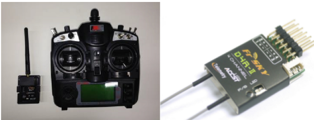
Fig. 3. FrSKY DJT Radio Telemetry (RF module, left of left figure), FlySky FH-TH9X Transmitter (transmitter body, right of left figure), and FrSKY D4R-II 4Ch Receiver (receiver, right figure)
