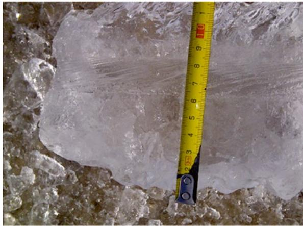
**Figure 7.15** Rime icing vane (Wareing 1999).
