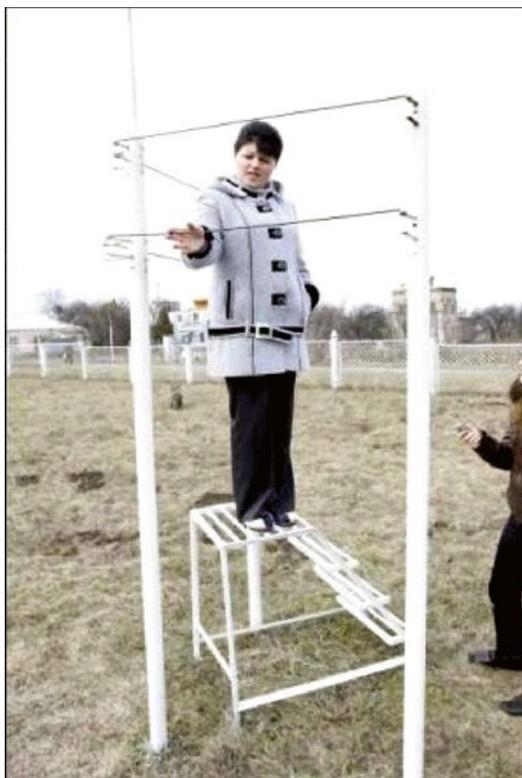
Some countries are using test spans, for instance in Iceland (measured since 1972) as shown in Figure 7.20 (Cigré TB 291).
