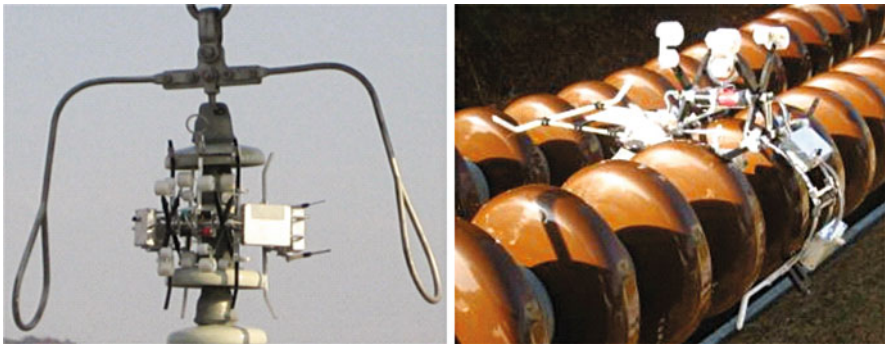
Figure 16.21 Live-line insulator inspection robot developed by KEPCO, 2010.
