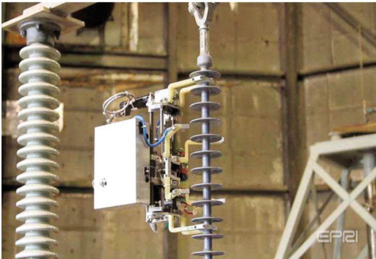
Figure 16.22 Technology demonstrator of the EPRI insulator crawling robot that is being investigated to replace the hand held operation.
