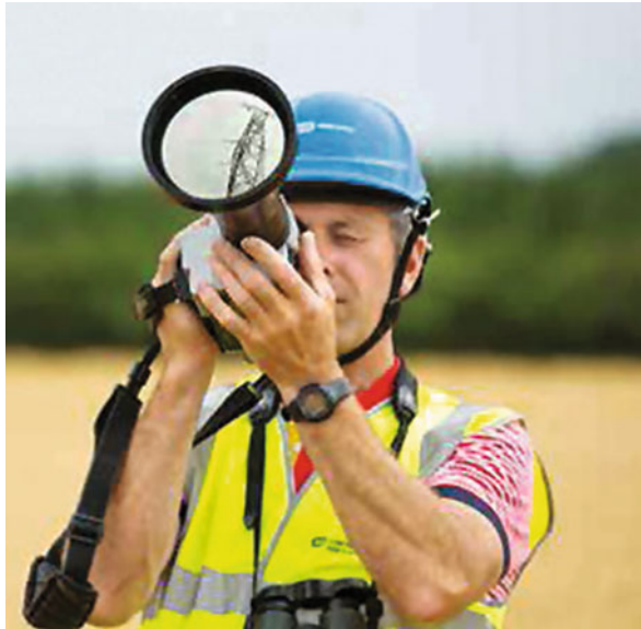
Figure 16.4 Thermographic inspection performed from the ground.
