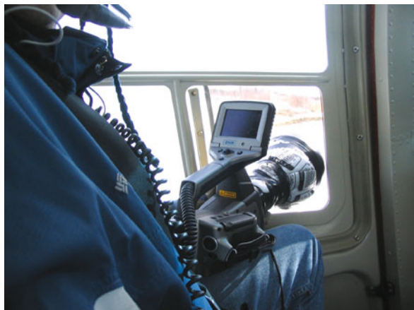
Figure 16.5 Thermographic inspection performed from a helicopter.
