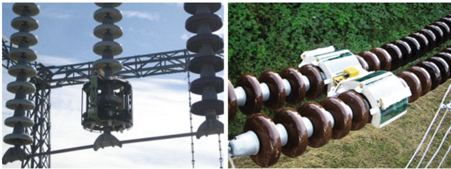
Figure 16.20 Live-line insulator cleaning robot developed by KEPCO 2006.
