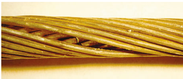
Figure 16.2 Broken Inner Conductors Strands.
