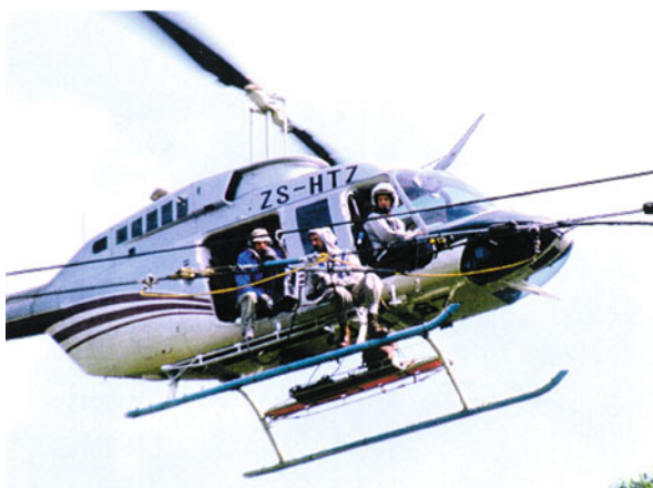
Figure 16.13 Changing 600 kV Insulator String using Bare Hand Method (Brazil).
